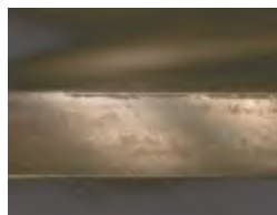
Relief face Flank wear 0.09 mm
