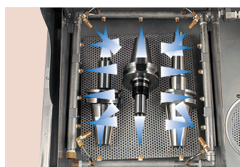
Automatic washing from 18 nozzles.
