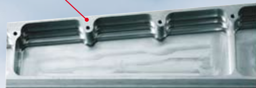
Geometrically milled, complex aircraft structure made of aluminum.
