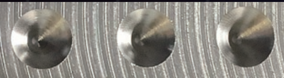
Good! Depth=2.4mm(0.2D) Step=0.6mm
