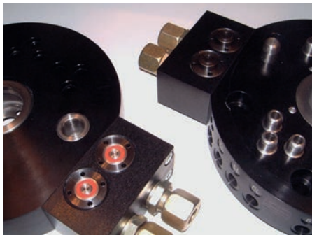
Coupling system for extrem low leakage hydraulic oil fed in tool changing modules of a robot. Therefore two hydraulic lines are coupled by threaded-body coupling elements (M24x1.5).
