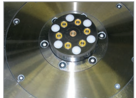
Coupling plate used for the transmission of hydraulic oil in the loading and unloading station of a fixture plate. The six coupling elements are coupled pressurized.
