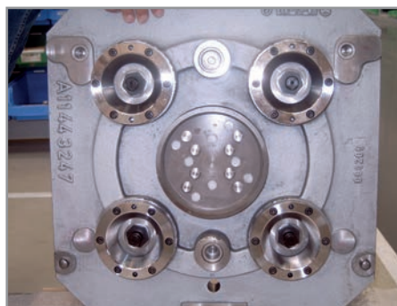
Coupling nipple plate in the fixture plate of a machine tool. The nipple plate is docked to the docking unit (figure above) and hydro-mechanically locked.
