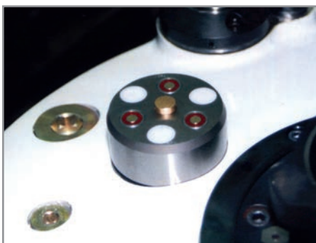
Triple coupling system for hydraulic oil fed in the fixture plate in a machine tool. The connection in the loading and unloading station is realized through the lowering of the fixture plate.
